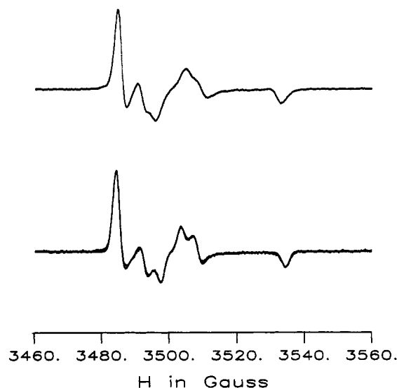
FIGURE 2: EPR spectra from [^{15}\text{N}, ^2\text{H}]\text{MTSL-S1} free in solution (top) and immobilized by precipitation in ammonium sulfate (bottom, dotted line). The spectrum from [^{15}\text{N}, ^2\text{H}]\text{MTSL-S1} free in solution is characteristic of a slowly moving randomly oriented spin probe. The spectrum from the immobilized probe is fitted (solid line) as described in the text (see Results, section A). Spectra were measured with a modulation amplitude of 0.5 G and a microwave power of 5 mW.
